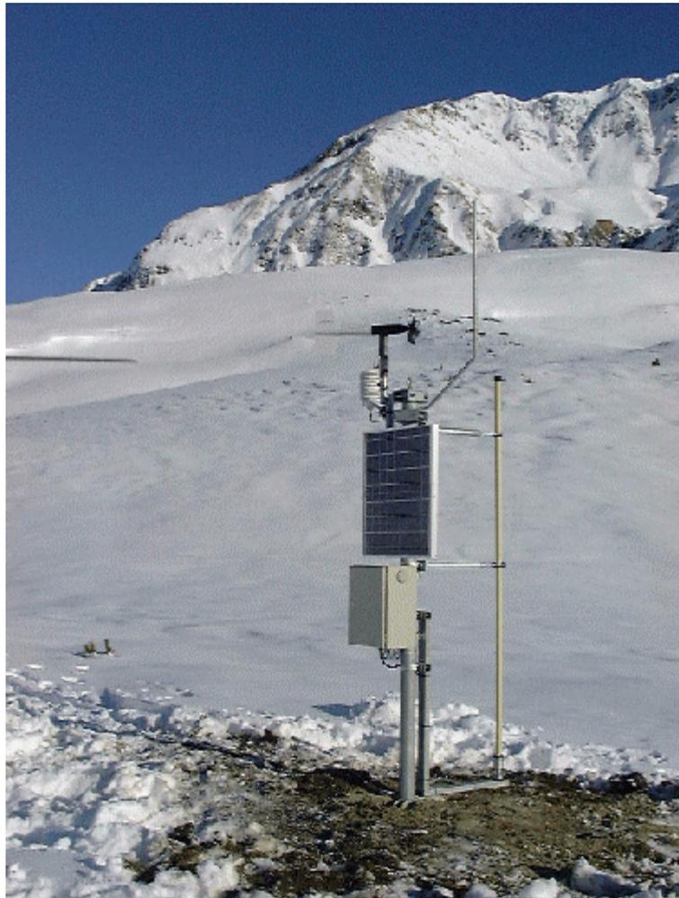
Standard Fcapt station Lukmanier. The station automatically alerts the road maintenance crew in case of snow transport. Measured parameters are: wind, wind direction, air temperature and blowing snow flux. Data and alarms are transmitted by radio or GSM.
