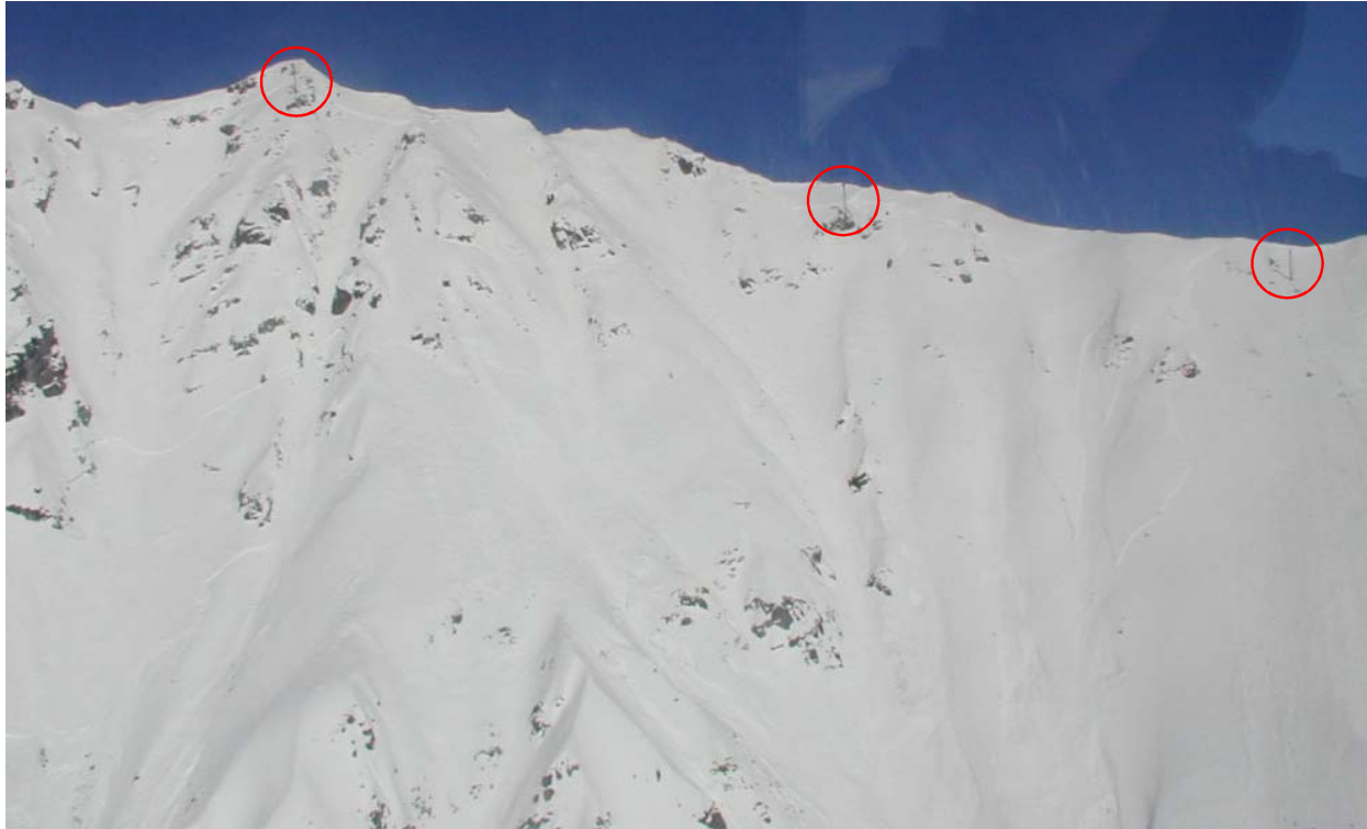
Figure 7: Part of the huge bowl of the Gonda release zone with 3 positions of avalanche towers.
